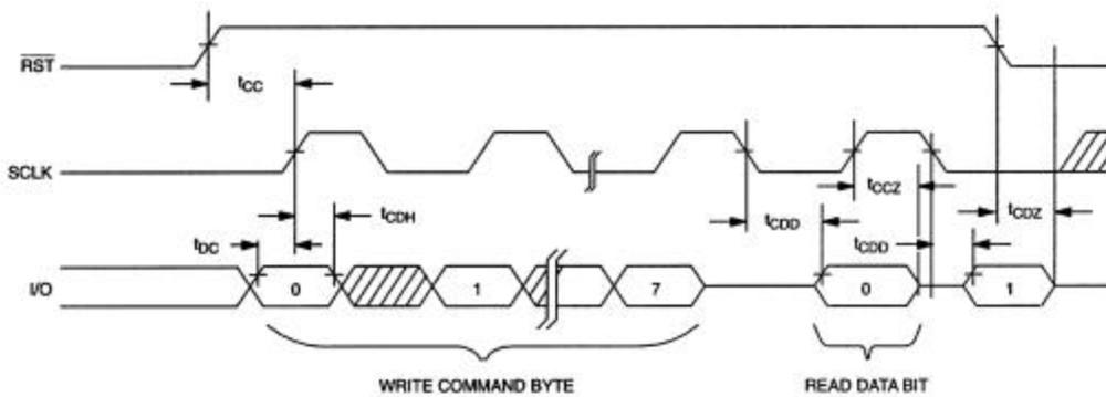
**TIMING DIAGRAM: WRITE DATA TRANSFER** Figure 6
