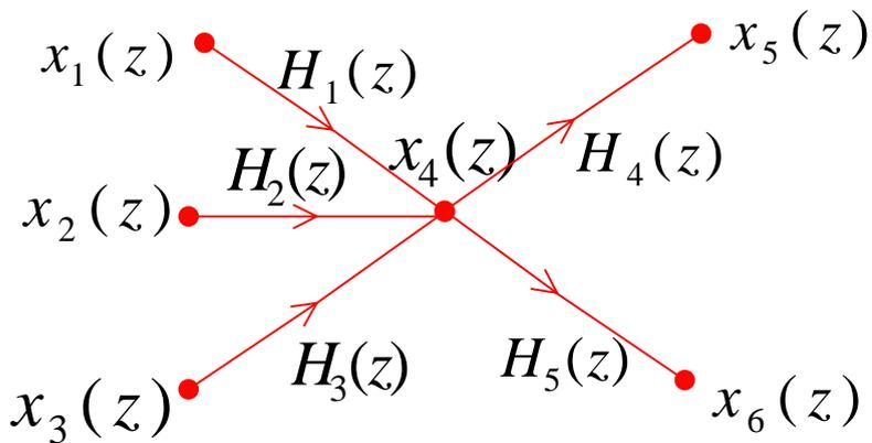
$$X_4(z) = H_1(z)X_1(z) + H_2(z)X_2(z) + H_3(z)X_3(z)$$
